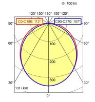
light sourceLEDwork equipmentwithoutconnected load22-26 V, DCpower consumptionenv. 28 Wluminous fluxapprox. 700 lmluminous efficiencyapprox. 25 lm/W
